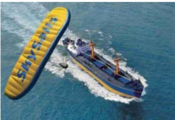
*SkySails, a concept to use wind power for commercial propulsion*
